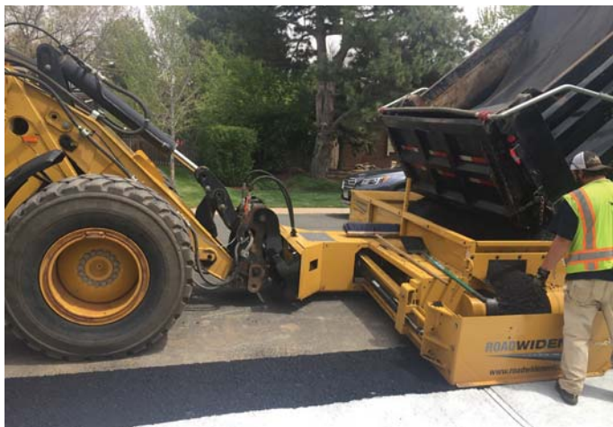
Road Widener attachments are designed to connect via a quick-connect coupler; however, with an adapter we can be added to any machine.
